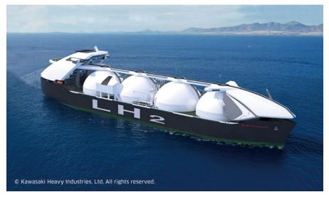
(Concept image of 160,000 m liquefied hydrogen carrier provided by Kawasaki Heavy Industries, Ltd.)
